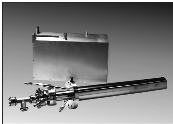
Figure 1. SVT Associates 4.5" (114mm) OD CFF RF Source shown with matching network. A smaller version which mounts on a 2.75" (70mm) OD CFF is also available.
