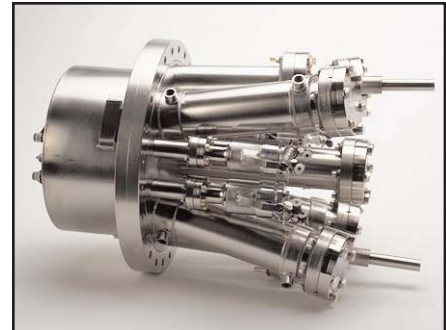
Side view showing rotary pneumatic cell shutters.
